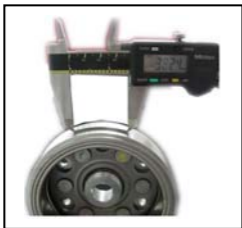
Gambar 4 : Mengukur Pick Up Pulser
