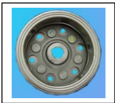
Gambar 2 : Fly Wheel (Magneto)
